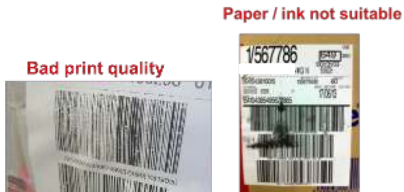
Figure 9-2 Examples of printing-related problems
